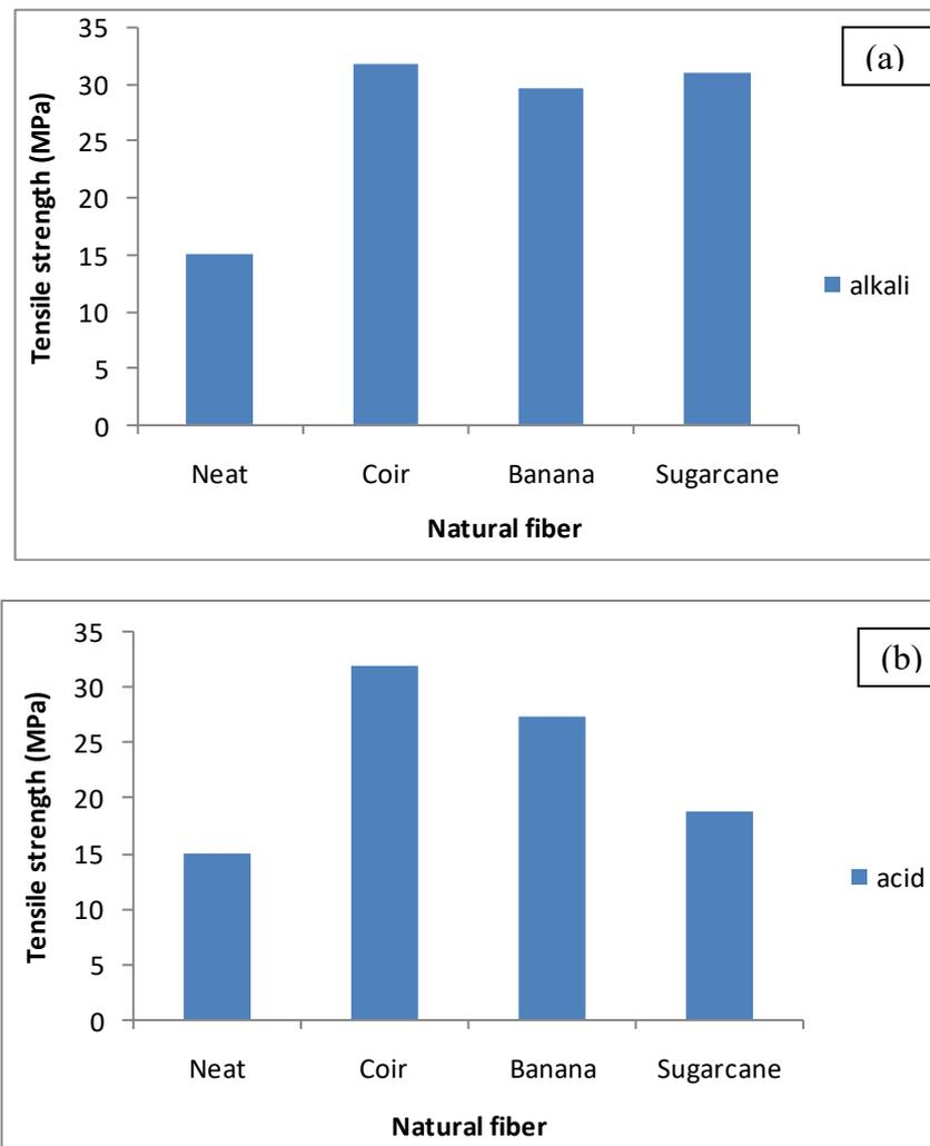
**Figure 1.** Tensile strength of the variation epoxy/natural fibers composites (a) alkaline treated (b) acidic treated.
