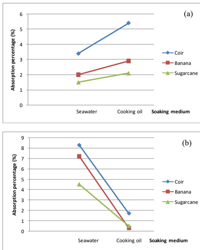
**Figure 2.** Swelling percentage for epoxy/natural fiber composites in cooking oil and seawater after 3 days (a) alkaline treated (b) acid treated.
